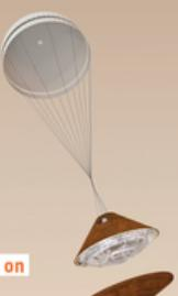
**Front shield separates, radar turns on**
