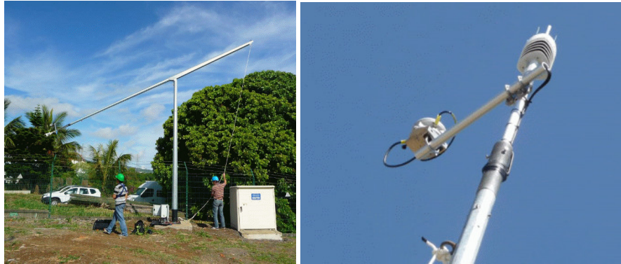
Fig. 7. 10-meter high foldable mast supporting a measurement station.
