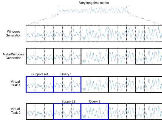
Fig. 1: Task design for a univariate time series, also applicable to multivariate time series. We omit the other channels and the respective target associated to every window for the sake of simplicity.
