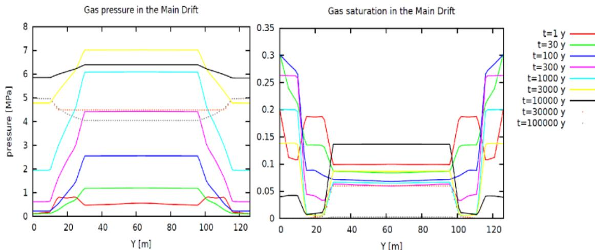
**Figure:** Gas pressure (left) and gas saturation (right) in the Main drift.
