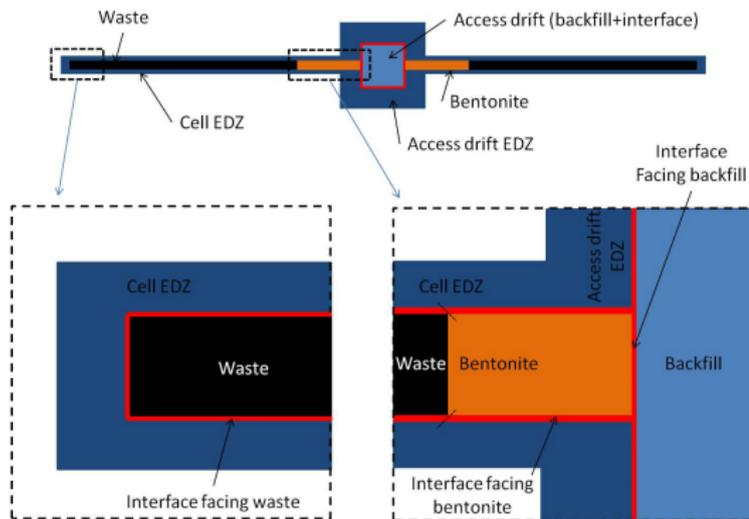
Figure: Schematic representation of the B-B' vertical cross section.
