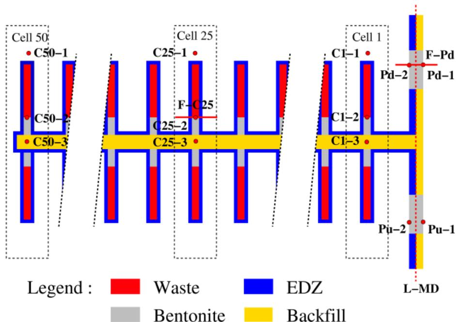
**Figure:** Definition of the points where results have been extracted, of the line L-MD and of the surfaces F-C25 and F-Pd.
