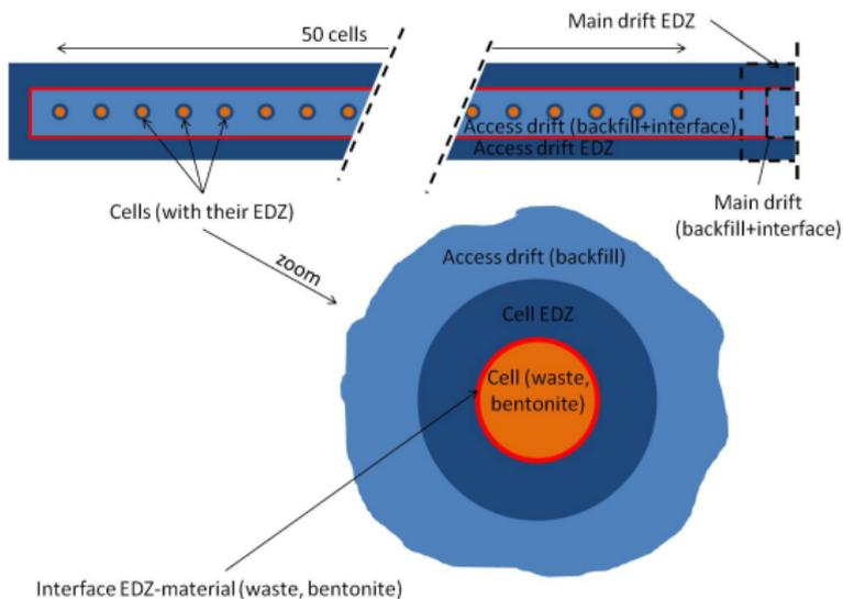
**Figure:** Schematic representation of the A-A' vertical cross section.
