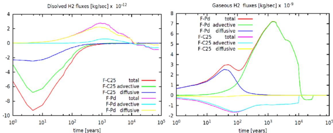
**Figure:** Dissolved hydrogen fluxes (Left) and Gaseous hydrogen fluxes (Right).
