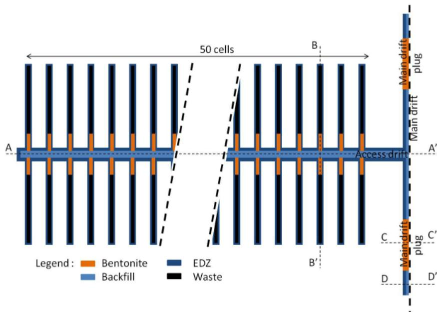
**Figure:** Schematic representation of the module to be simulated. Definition of the A-A', B-B' cross sections.
