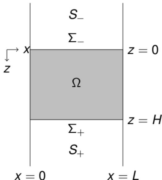
A cartoon illustrating the parts of  $S$ . One period of the grating occupies  $\Omega$ . In  $S_-$  and  $S_+$  the parameters are constant.
