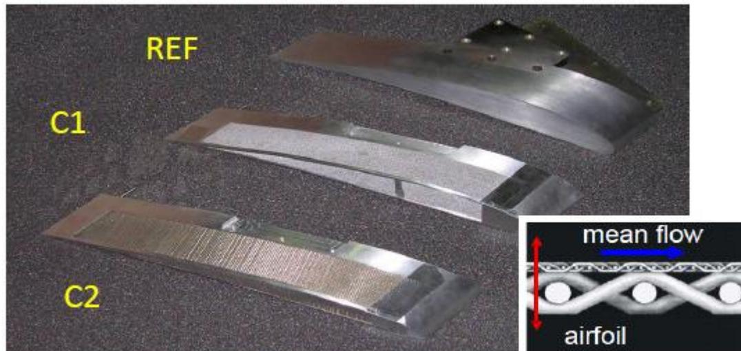
*Coin de volet poreux OPENAIR (DASSAULT-EADS IW)*
