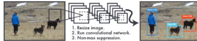
Figure 1: The YOLO Detection System. Processing images with YOLO is simple and straightforward. Our system (1) resizes the input image to 448 \times 448 , (2) runs a single convolutional network on the image, and (3) thresholds the resulting detections by the model's confidence.
