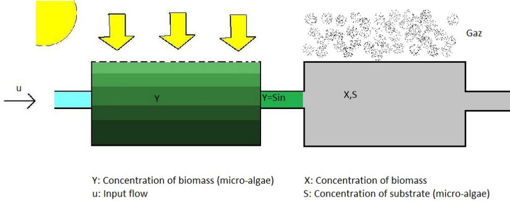
Figure 8: A dual tank bioreactor for converting microalgae into methane
