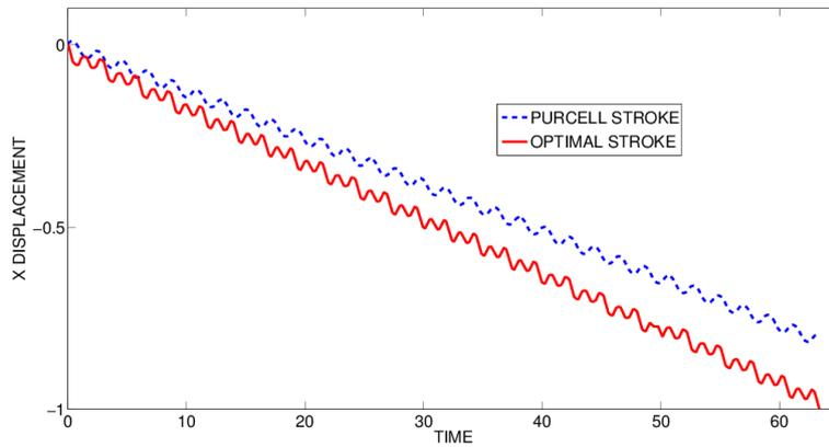
Figure 23: **purcell**: comparison of Purcell and optimal strokes
