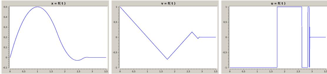
Figure 1: **fuller**: state  $x, v$  and chattering control  $u$
