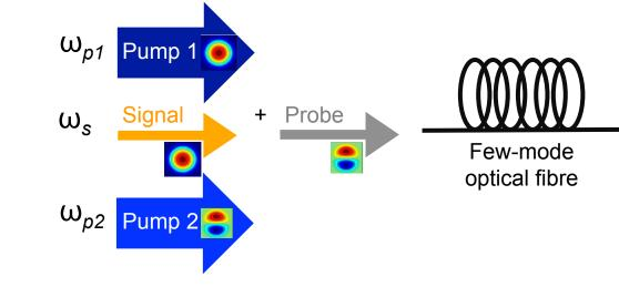
Two distinct IM-FWM processes simultaneously occur, leading to interferences that can **inhibit or enhance the signal amplification** (depending on the phase of the input signal wave).
