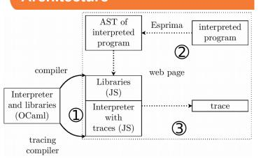
The JavaScript interpreter is written in Ocaml. It is derived from the interpreter extracted from the JSCert project that was written in Cog. It is compiled into JavaScript so that it can be embeded in the web interface (①). The source code is converted in a specific data structure called Abstract Syntax Tree (2). The interpreter takes it as input and produces the program execution trace (③).
