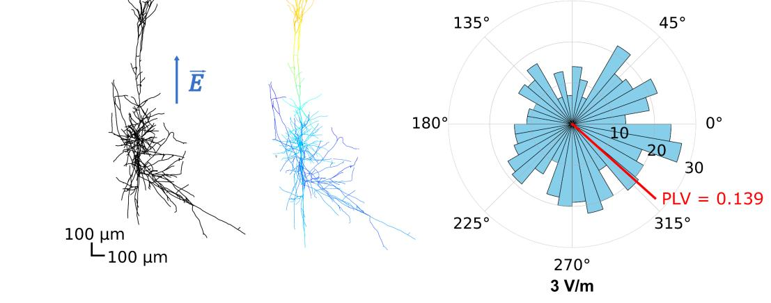
→ Quantification of electric fields effects on the phase coherence of neuronal firing.
