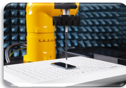
State of the Art: Free-space measurements in vicinity of mmWave device under test
