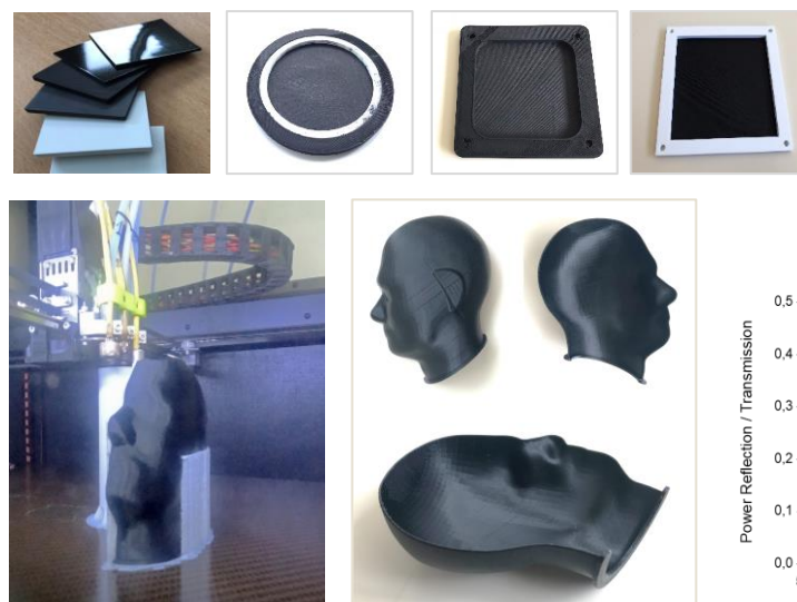
Fig. 1. The first 3D-printed reflectivity-based phantoms (flat and 3D-shaped) reproducing the EM reflection coefficient of the human skin in FR2 band for both TE/TM polarizations.
