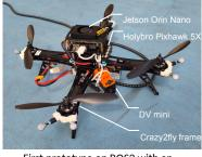
First prototype on ROS2 with an event camera and a Jetson board
