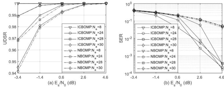
Figure 12: N-BOMP and ICBOMP performances for  $\alpha = 8$  antennas,  $N = 80$  nodes,  $N_{a \max} = 30$  iterations, the data size  $d = 124$  symbols and the message length  $m = 620$  symbols. [30]
