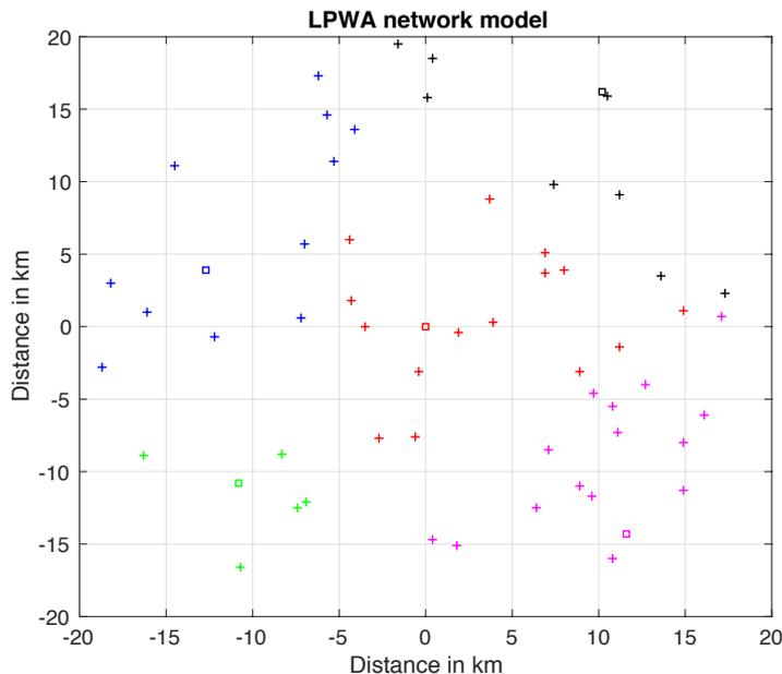
Figure 1: LPWA network model: each sensor is connected to the closest collector on which the average received power is the best. The sensors nodes are illustrated by + and the collectors by a square. The typical cluster contains the red nodes.
