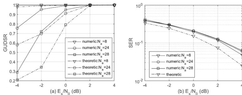
Figure 11: N-BOMP numerical and theoretical performances for  $\alpha = 8$  antennas,  $N = 80$  nodes,  $N_{a \max} = 30$  iterations, the data size  $d = 100$  symbols and the message length  $m = 500$  symbols.[30]
