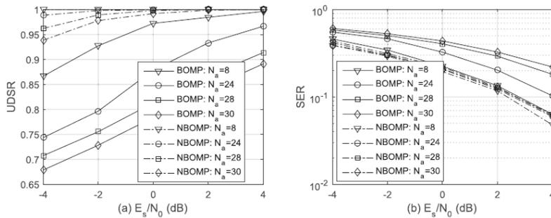
Figure 10: BOMP and N-BOMP performance for  $\alpha = 8$  antennas,  $N = 80$  nodes,  $N_{a \max} = 30$  iterations, the data size  $d = 100$  symbols and the message length  $m = 500$  symbols.[30]
