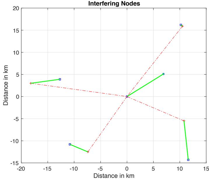
Figure 2: There is only one interfering node per cell. The useful signals are illustrated by the green line. The interfering signals are illustrated by red dashed lines. The set of interfering node can be approximated by an heterogeneous PPP with intensity  $\lambda(x) = \lambda_b(1 - e^{-\lambda_b\pi|x|^2})$ .
