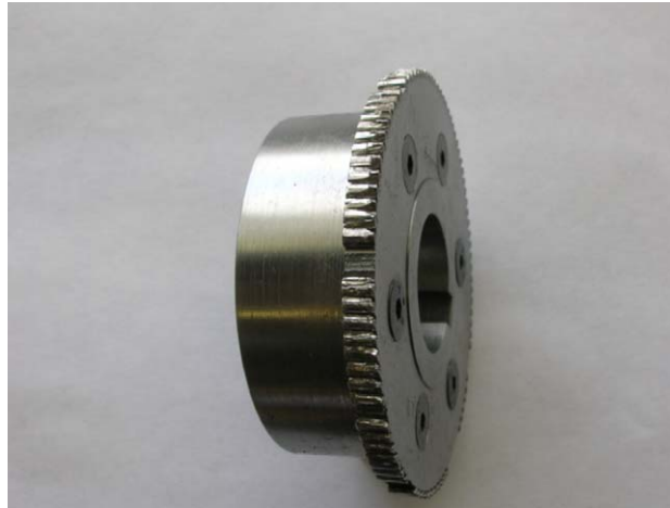
Fig. 14. Photo of the damaged gear at the end of the experiment.
