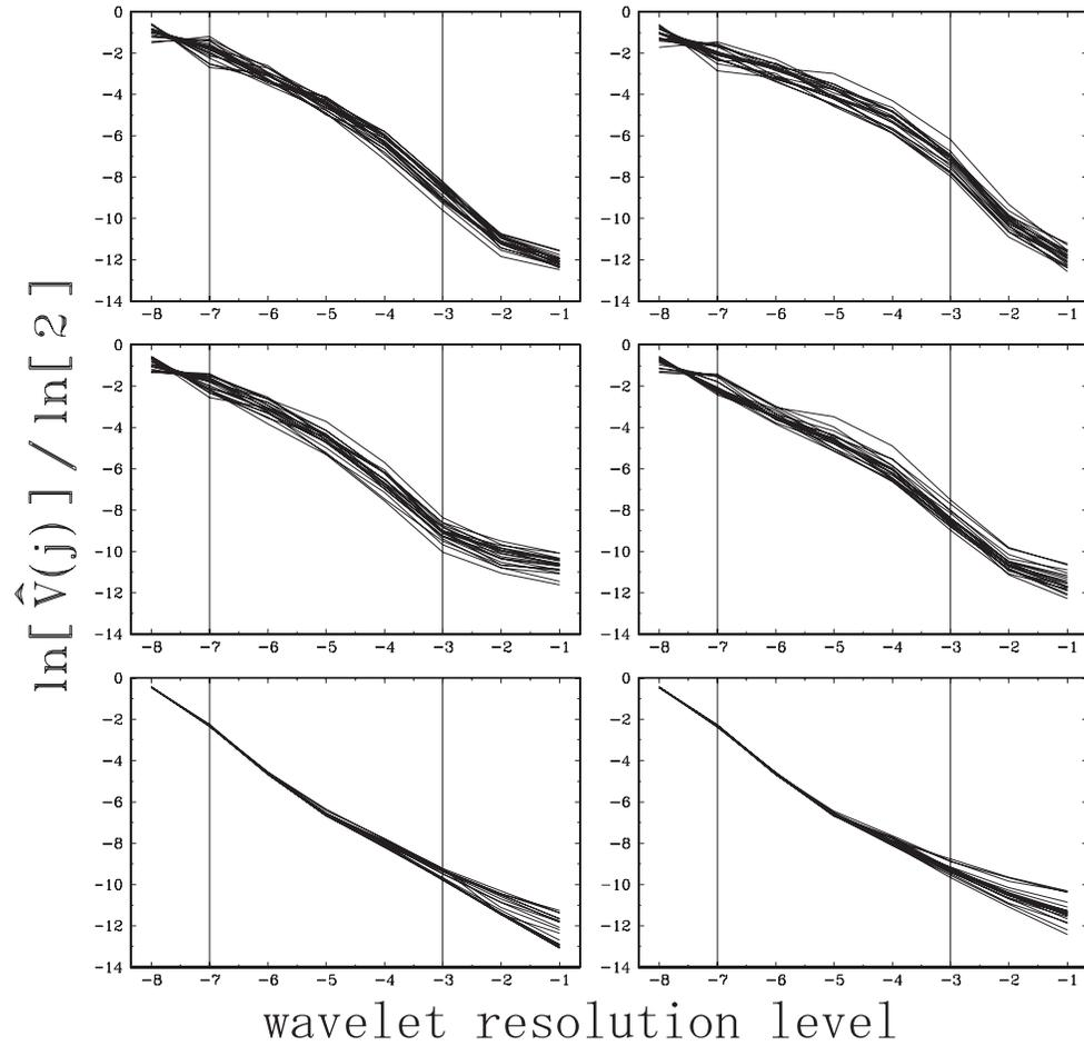
Fig. 6. Evaluation of Hurst exponent for laser beam  $x$ -coordinate (left column) and  $y$ -coordinate, for hard (top), soft (center) and normal (bottom) turbulence. The vertical lines represent the scaling region used in the evaluation of  $H$ .
