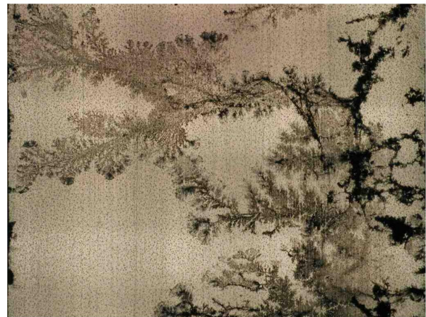
Fig. 2. Original image of a dendrite grown from immersion silver.
