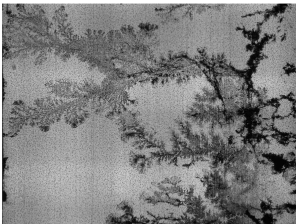
Fig. 4. Grayscale image (8 BPP) of a dendrite grown from immersion silver.
