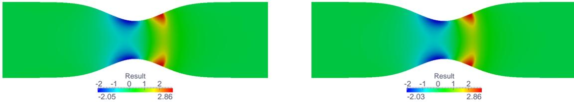
Figure 7.10: Bedload evolution at  $t = 10$  h for implicit solutions with  $CFL = 100$  (left) and  $CFL = 1000$  (right) using Mesh 2.
