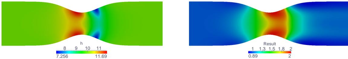
Figure 7.6: Height of the flow (right) and modulus of the velocity (right) at  $t = 10$  h for implicit solutions with  $CFL = 100$  using Mesh 1.
