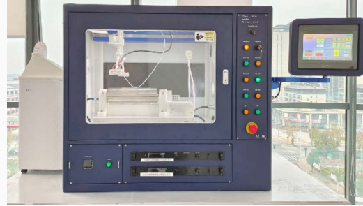
Fig. Device used to generate the EPs_Explore_1d8k dataset: TL-PRO electrospinning machine from Shenzhen Tongli Micro-Nano Technology Co., Ltd. Device size: 1100 mm × 730 mm × 950 mm.
