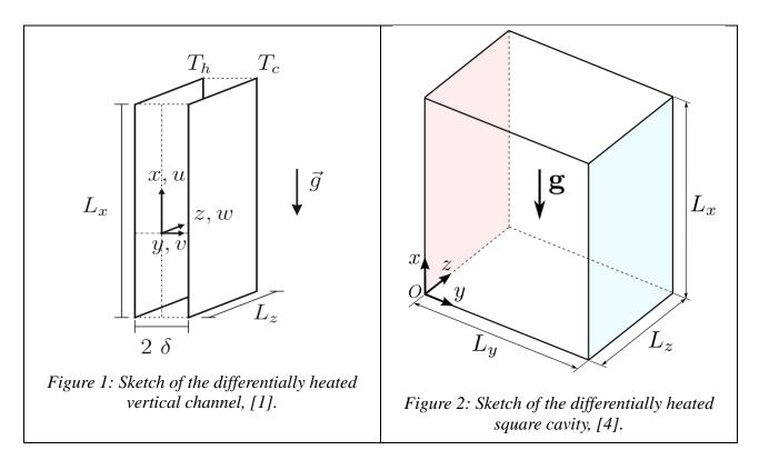
Regarding turbulent channel flows, a large number of studies focus on forced convection or natural convection in a horizontal channel (Rayleigh-Benard convection). For a horizontal channel, production / destruction of turbulent kinetic through buoyancy effects involves the wall-normal heat flux. For a vertical channel, buoyancy effects on turbulent kinetic energy involve the wall-parallel heat flux. This fundamental difference can be of prime importance.
