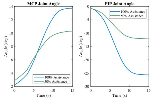
Fig. 2. Validation of assistance modulation during implementation of the TA intervention. The plots show the angular positions of the robots MCP and PIP joints during actuation at two different assistance levels.
