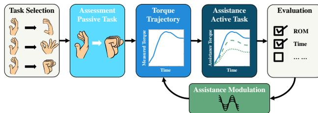
Fig. 1. An overview of the work flow for the task assistance (TA) intervention. After hand pose selection, the Maestro hand exoskeleton performs a passive task assessment and measures the robot joint torque trajectories necessary to reach the selected hand pose. Next, the user is asked to reach the hand pose during the active task, and the Maestro hand exoskeleton modulates the level of task assistance throughout the therapy session with the goal of encouraging increased user effort over time.
