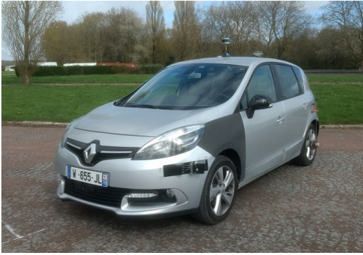
Fig. 1. The perception vehicle used : two ibeo LUX, the VLP16, GNSS antenna and the precision odometer are visible
