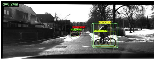
Figure 10. Road scene image overlaid with objects recognition and distance estimation results achieved by proposed DisNet and by stereo-vision based HiSpe3D method [17]
