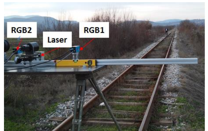
Figure 8. Field tests performed on the straight rail tracks; Test-stand with the SMART sensors viewing the rail tracks and an object (person) on the rail track
