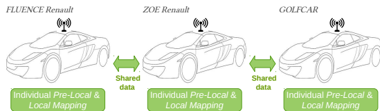
Fig. 1. Scheme of our CoMapping System considering a decentralized case
