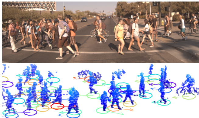
Fig. 1. Association and tracking of pedestrians is challenging in dense, urban environments. We propose a real-time learned association and tracking system with IMM filtering that incorporates LiDAR + camera modalities and show improvements on the task of both association and state estimation.
