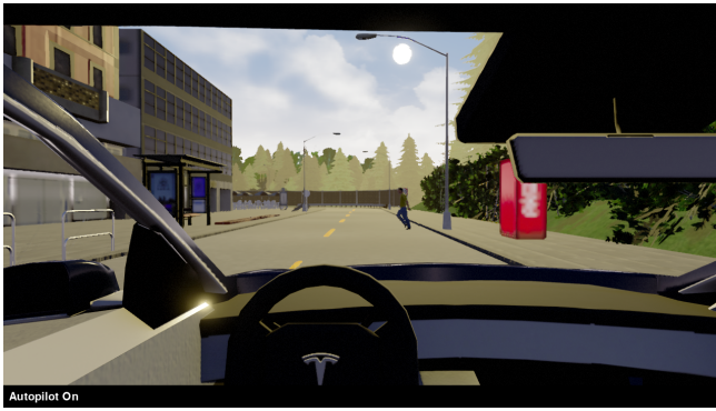
Fig. 4. Screenshot of the simulation in one of the emergency scenarios. The pedestrian is stepping down to the road ahead the vehicle from behind a vending machine; the weather is clear with good visual conditions and there is no traffic on the road.
