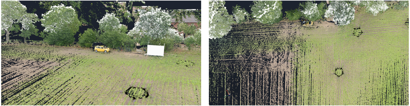
Fig. 5. Colored 3D point cloud of the data collected with the terrestrial laser scanner of the AROX robot. Color values are derived from the integrated RGB camera. Annotation with hyperspectral data is also possible.
