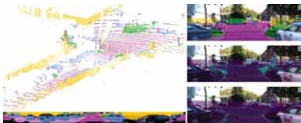
Fig. 2. A sample qualitative result. At the bottom, the range-view image of the network response is shown. The top camera image on the right shows the projected segments whereas the middle and bottom images depict the projected epistemic and aleatoric uncertainties, respectively. Note that the lighter the color is, the more uncertain the network becomes.
