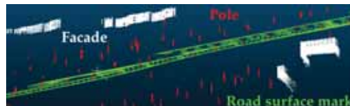
Fig. 1. The semantic point cloud map (SPCM) used in this study contains a sparse point cloud with only three kinds of static semantic features, which are poles, facades, and road surface marks.
