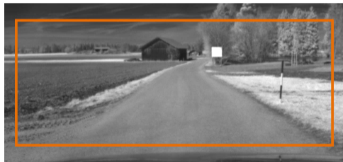
NIR image from a Basler acA1300-60gmNIR with a 765nm longpass filter.
