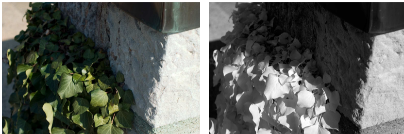
A RGB/VIS image of vegetation and a Near-Infrared (NIR, 770-1100nm) capture of the same scene (from [1]).
