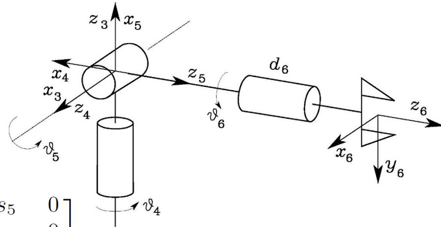
$$A_4^3 = \begin{bmatrix} c_4 & 0 & -s_4 & 0 \\ s_4 & 0 & c_4 & 0 \\ 0 & -1 & 0 & 0 \\ 0 & 0 & 0 & 1 \end{bmatrix}$$
