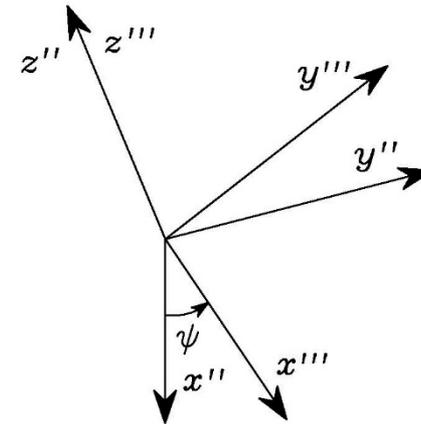
$$R(\phi) = R_z(\varphi)R_{y'}(\vartheta)R_{z''}(\psi)$$
