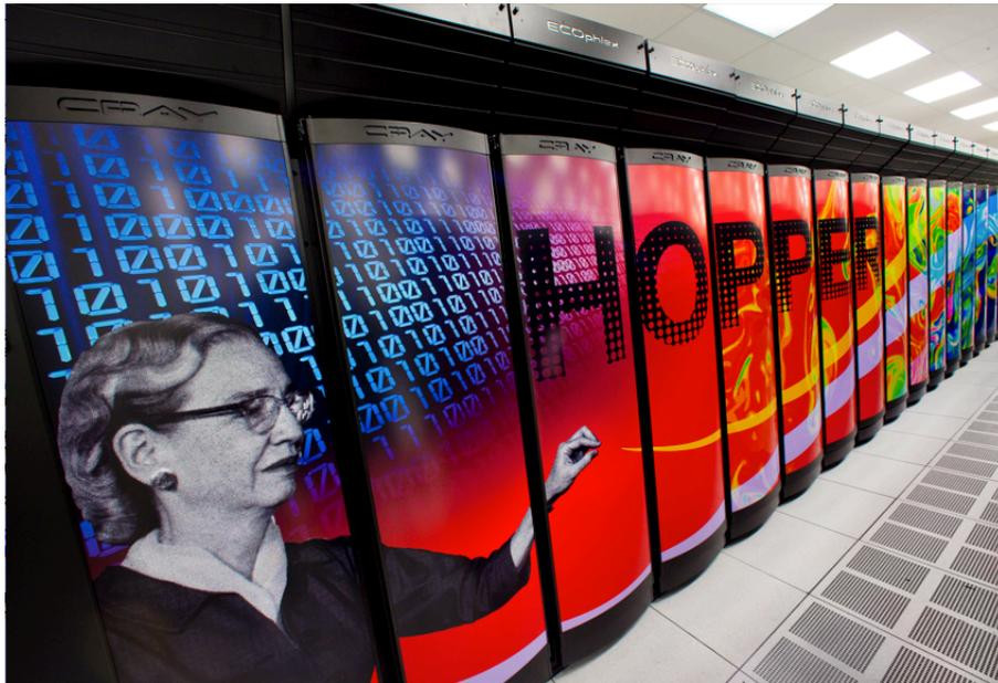
NERSC Hopper - a 1.28 petaflops/sec Cray XE6 with 6,384 compute nodes (24 cores/node, totaling 153,216 cores) and 212 TB of memory
