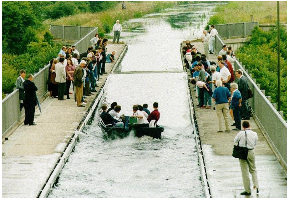
Experimental reproduction of the Scott Russell solitary wave in a water canal at Heriot-Watt Univ. in Scotland (12 July 1995). Re-creation of the famous 1834 'first' sighting of a soliton or solitary wave by John Scott Russell on the Union Canal near Edinburgh.
