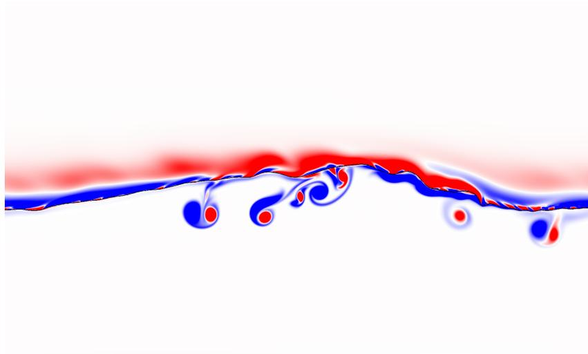
Figure 1 : Vorticity field above and under water during a spilling breaking with dipoles in deep water.
