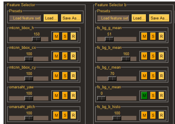
Figure 5: VACE loss function feature adjustment user interface. Features can be muted, solo'd, and have their weights adjusted, affecting the loss function summation.
